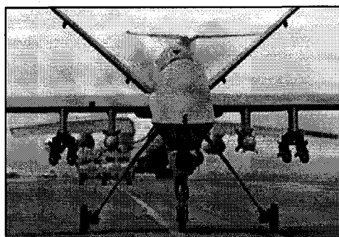
A fully armed MQ-9 Reaper (Group 5 UAS) taxis before a mission in Afghanistan. The MQ-9 Reaper provides persistent surveillance and target engagement capabilities to warfighters in Iraq and Afghanistan.
