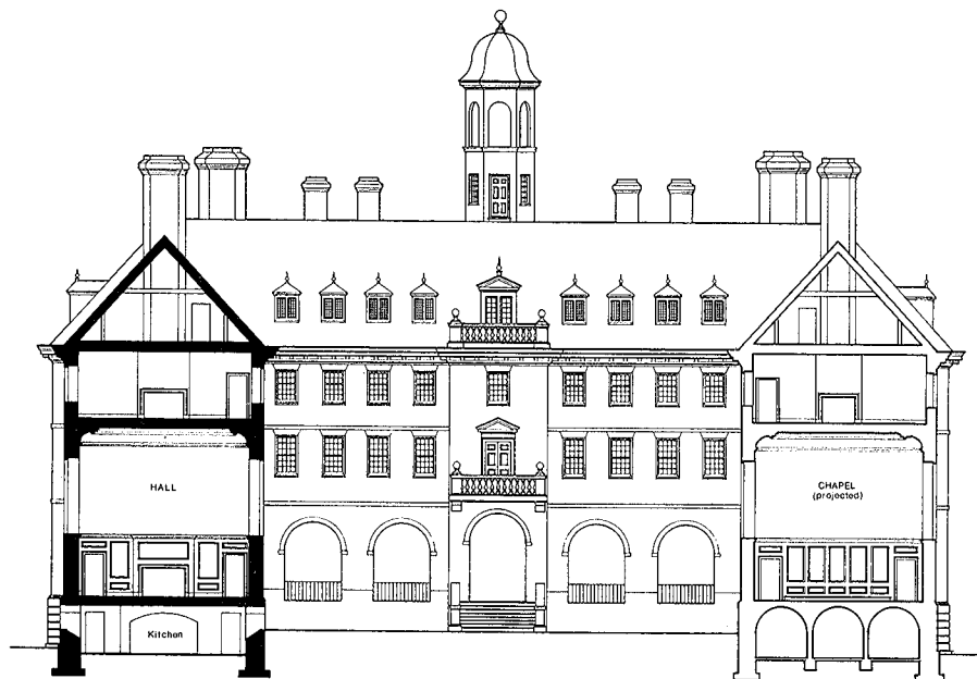
Figs. 24c–d. William S. Pavlovsky, North Elevation and West Elevation with Sections, The College of William and Mary (first building, 1695–1699) , drawings, 1988.
