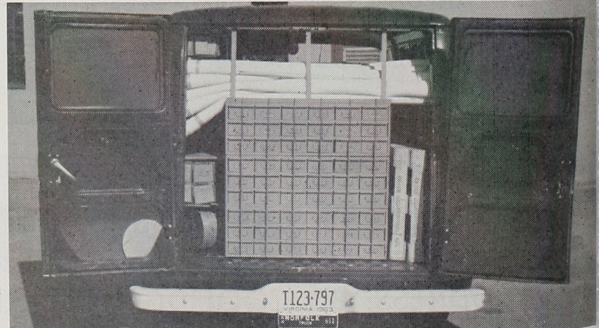
REAR VIEW of parts truck shows drawer arrangement and space which provides for larger supplies.
