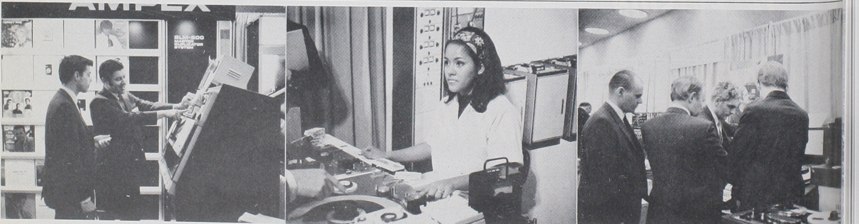
Ampex Stereo Tape engineering manager Marty Ehrlich proudly demonstrates the model BLM-200 master duplicator with vacuum bin to Ed Adlum. Ehrlich controls the Ampex duplicating operation in Elk Grove Village, Ill., turning out cartridges and cassettes under the Ampex label for consumer sale. At Elk Grove, Ehrlich utilizes 20 slaves duplicators with each BLM-200 master for cassettes, and ten slaves for the cartridges.
