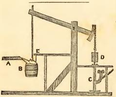
The plan and description of the machine represented in the engraving is copied from the Domestic Encyclopedia. It is a simple and valuable contrivance for making use of the power to be derived from a fall of water, when that power is too insignificant to justify the erection of a common water wheel.
