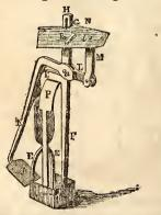
It may be used to good advantage without the wheels and lever, by having attached to it a piece of wood two set long, with handles, as represented in the small cut. It cuts a ditch smooth on the sides and bottom.
