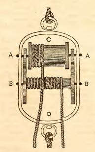
Mechanic, and represents an apparatus admirably adapted for the hoisting of ponderous bodies. It is thus described. Two horizontal axles with pivots at the ends, A, A, and B, B, have their bearings in an iron strap which has an eye at C, at the top, and another D, at the bottom. On the axle A, is a drum, round which is coiled a small rope; and at each end of the drum is a small pinion. On the axle B, are two geer wheels, the teeth of which work in those of the
