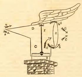
We present above, a sectional view of Mr. Espy's Invention for ventilating Ships, Hospitals, Prisons, Mines, Cisterns, Vats, Sinks, &c.-also for producing a strong draft in Chimnies, flues of Steamboats, Locomotives, &c.
