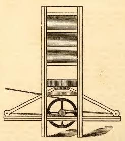
Messrs. Editors,—The above cut is an illus- | each side to keep it on the track of the railway. tration of the patent lever railway press, lately invented by William C. Van Hosen, of Catskill, Greene county, State of New York. The frame and box of this press are like those now in use. It will be seen by the cut, that the lower pannel is left out to show the follower or moveable bottom of the box with the end of the lever attached thereto. At the lower ends of the levers
