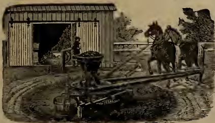
Triple Geared Feed Mill and Power Combined.
