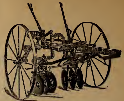
Bement Disc Cultivator, with 6 or 8 Disc. Built entirely of steel, steel forgings and malleable iron. The most simple and easiest adjusted cultivator on the market to-day. Write for circulars and testimonials.
