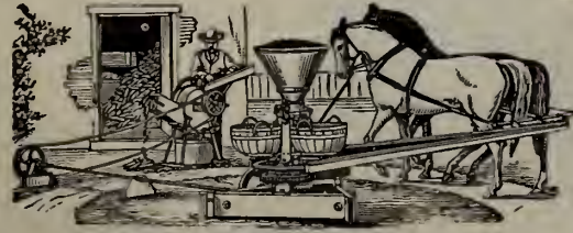
Scientific No. 8 used as a power, including 15-foot tumbling rod, two rod rests, and pulley, either 18 by 4 inches, 20 by four inches, or 24 by 4 inches. Tumbling rod makes 58 revolutions per minute. Fast enough for running feed cutters, shellers, wood saws, etc.
