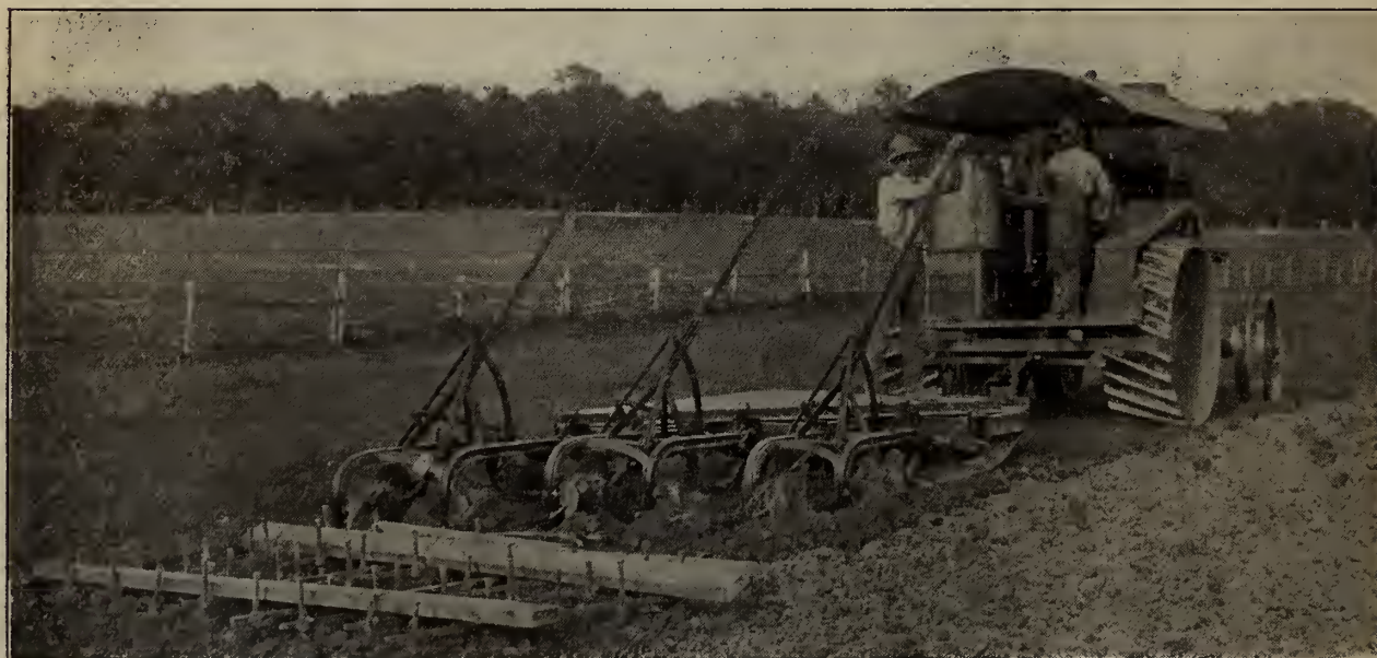
Six bottom John Deere Big Engine Gang in operation on Mr. G. H. Morrison's farm, Fredericksburg, Va.
