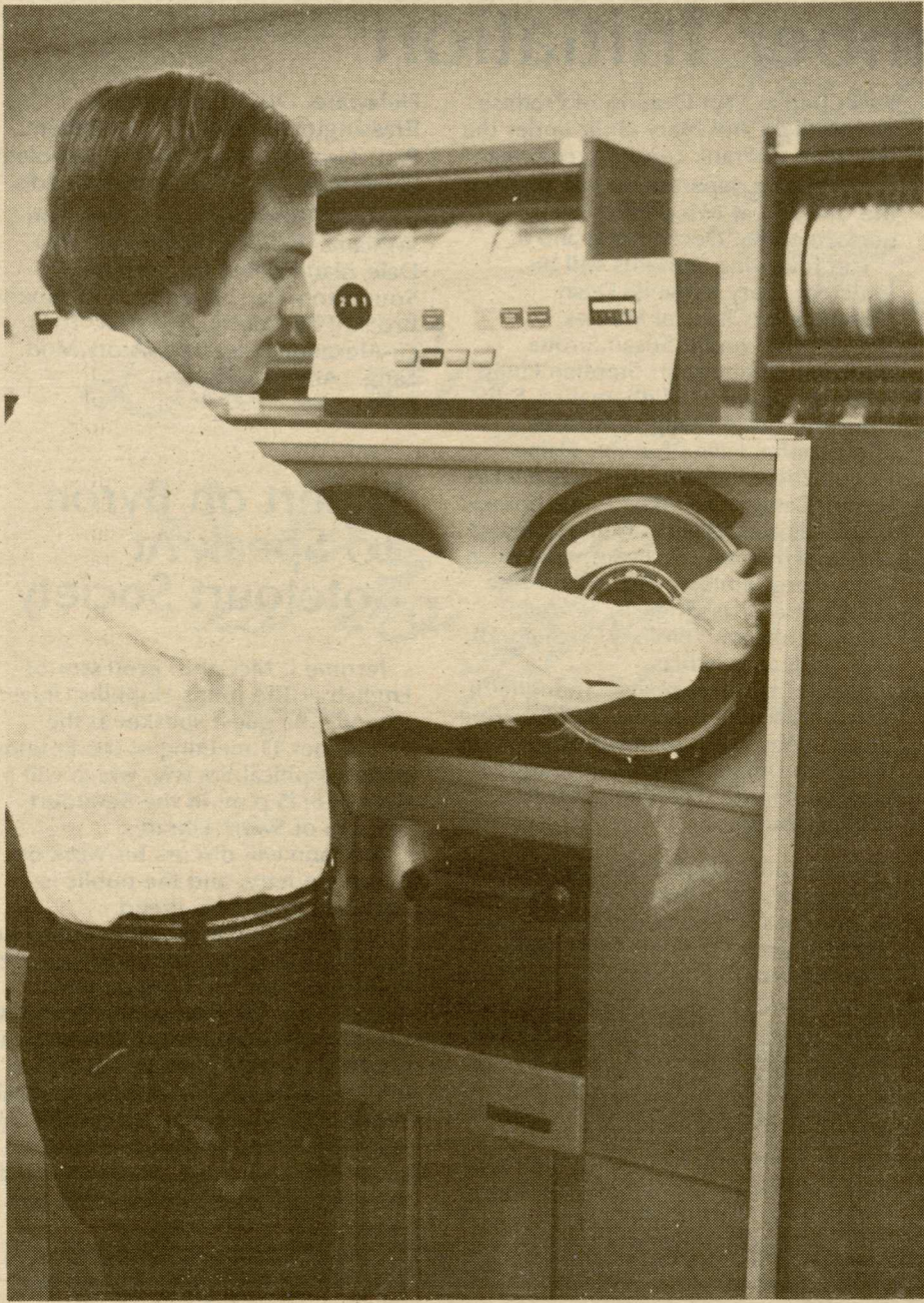
JOHN PEACH, operations supervisor, loads tape into the computer science center's new IBM system 370, model 158.
