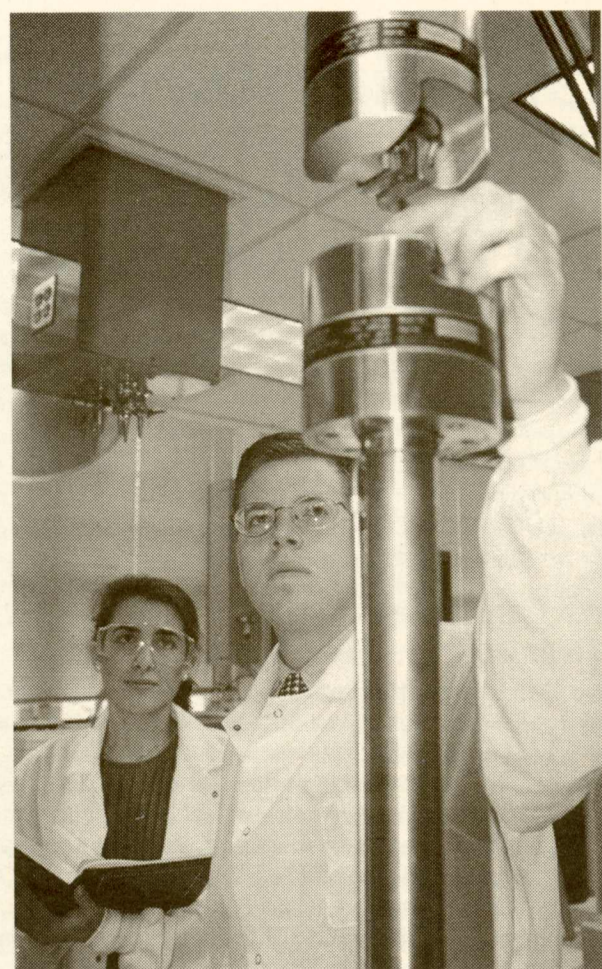
Seniors Pam Argiriadi and Andrew Meyer use the MTS (Material Test System), which tests the mechanical properties of polymers, such as stress and strain, and how these properties change as samples age.
