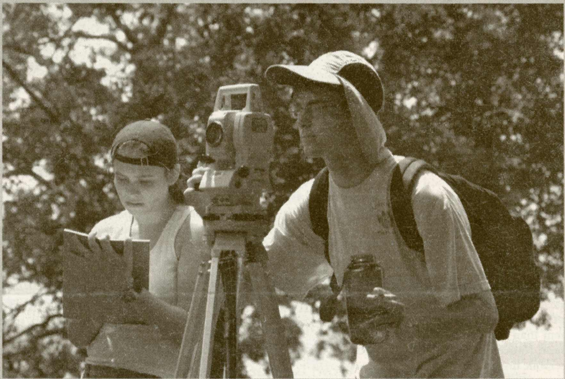
At the end of a day's dig, Cyndi Vollbrecht ('05) (l) and Matt Whalen ('06) use the "total station" to measure the amount of dirt sifted and removed from various excavation units.
