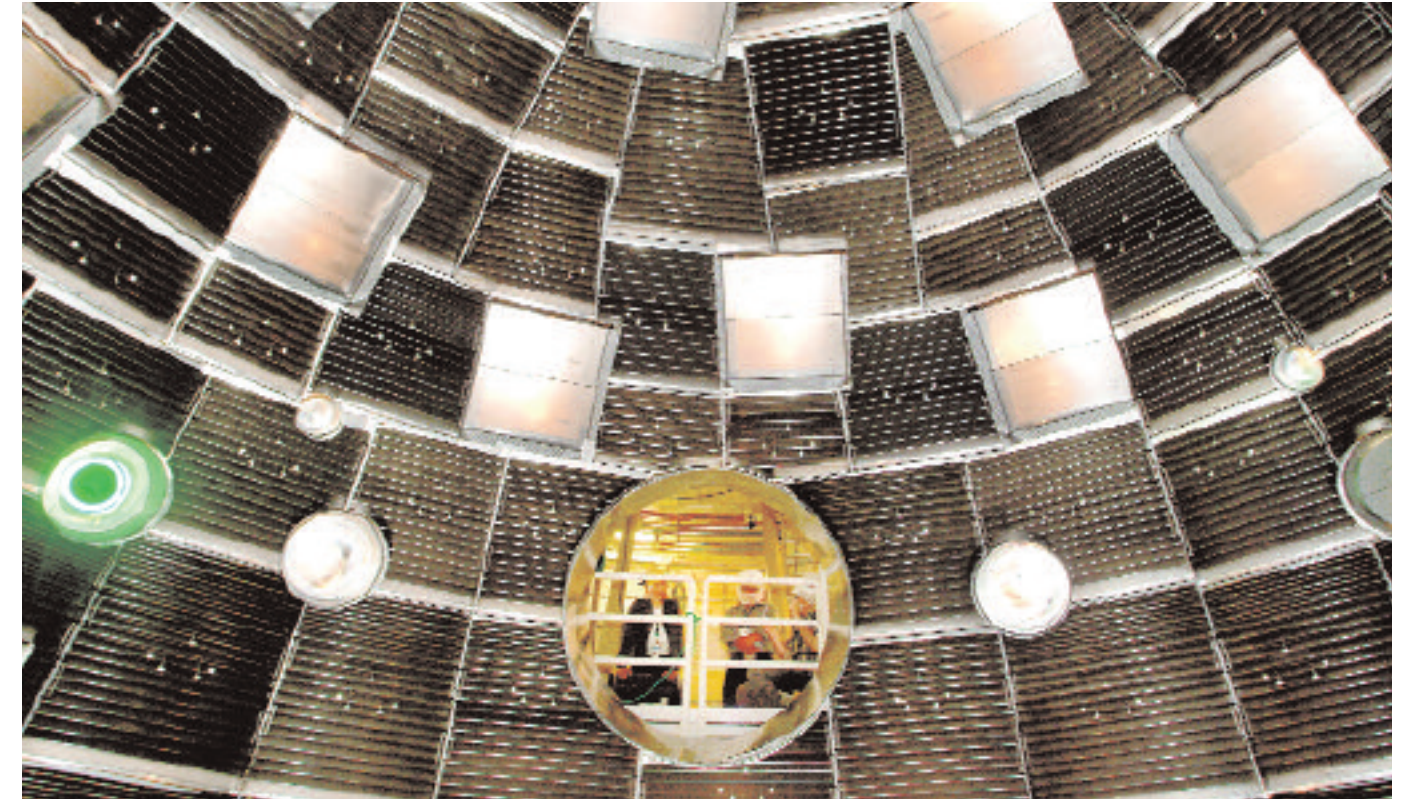
Inside the National Ignition Facility (NIF): Featuring 192 powerful lasers, the NIF has a diverse array of applications. When complete, it will be used to test weapons simulation codes, help study the evolution of stars, and research nuclear fusion energy.
