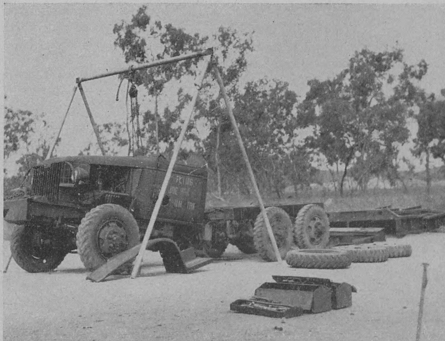
A view of the 6x6 cargo truck, airborne, broken down and ready for air shipment.
