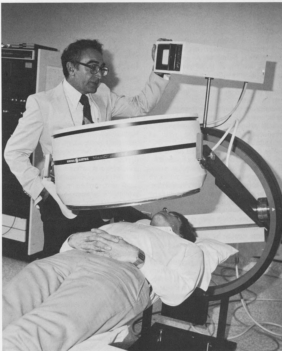
Gamma cameras such as the one pictured above at the San Diego Veterans Administration Hospital are used to detect radio-labeled antibodies which have localized to tumor sites in vivo .
